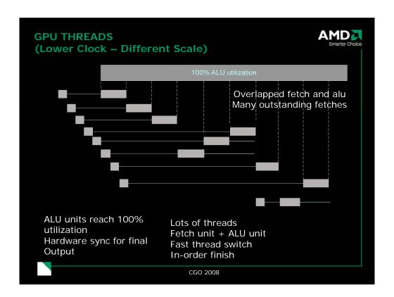
The big bar at the top shows when the float units are running. It is 100% active if there are enough threads
