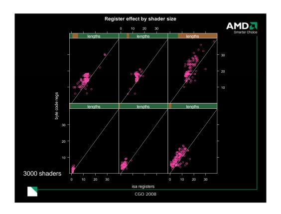
Shows the delta in registers, hIsI thinks the machine has vector registers and it does, so hIsI does an ok job, I split the 3000 shaders into 6 groups by length Smallest are lower left, biggest are upper right (lots of small one not so many large ones)
