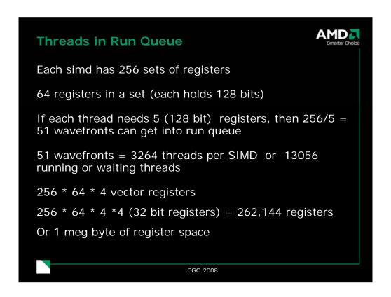
A thread is one pc/one group of registers, a wavefront is 64 threads
