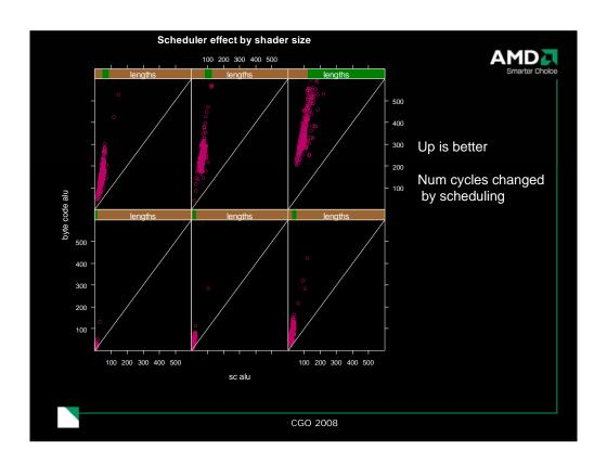
Here we have the same 3k shaders hlsl thiinks it is vector machine but is actually 5 way vliw, so the vector assignment does not work well
