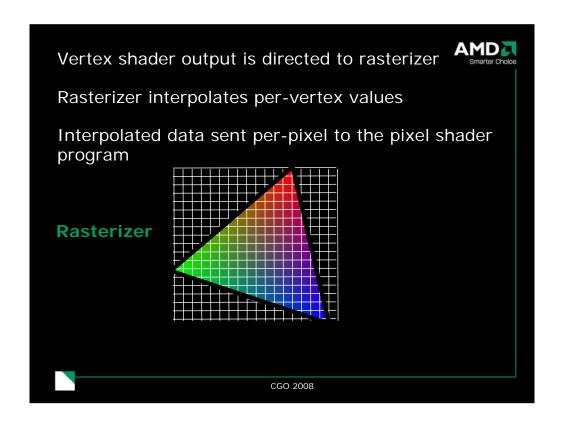
Each box in the grid gets its own thread, thread count is determined by hardware not by app, bigger screen means more threads
