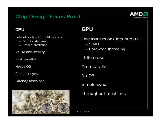
The main difference is that gpu's use multi-threading to tolerate latency, each time you wait for a read, just start another thread, This works if there are lots of threads
