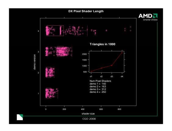
Box and whisker plot of shader length, box is ½ std div around mean, line is 1 and 1/2, outliers after this, size of max shader is growing, more control flow, Inside graph is the max triangles in 1000 triangle units so the highest value is 2 million, number of shaders is the count, time or chip version is going up d1 d2 d3 d4 are the demo numbers
